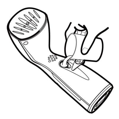
Figure 9 – Tank filling
