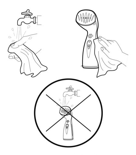
Figure 12 – Cleaning the device housing
